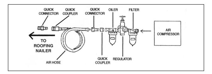
**Note:** To connect this tool, we recommend you use Air Plug (83, not included). For smoother operation and to extend the life-span of the tool, put 3-5 drops of pneumatic tool oil in the attached Air Plug (83) before each use.
